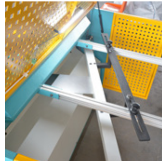
Standart Açılı Arka Dayama Standard Angle Backgauge
