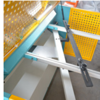
Standart Açılı Arka Dayama Standard Angle Backgauge
