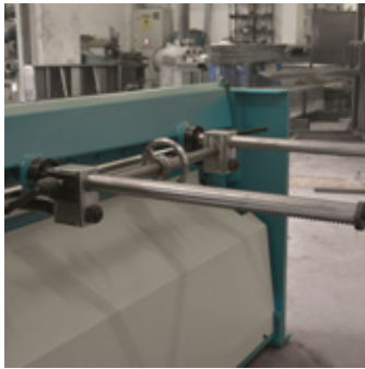
Standart Arka Dayama Standard Miter Backgauge
