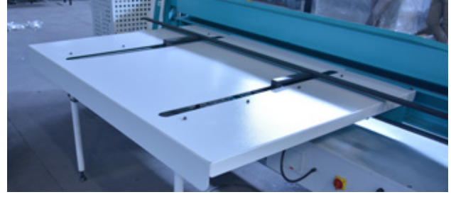
Motorlu Geniş Arka Dayama Bölgesi 750 mm Motorized Large & Stable Table for Motorized Backgauge 750 mm
