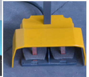
Elleri Serbest Bırakan Ayak Pedalları Handsfree Footpedal Operation for Clamping and Bending
