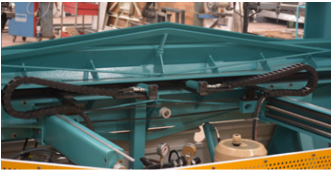
1 Otomatik + 1 Eksen Manuel Arka Dayamalar 1 Automatic + 1 Axis Manual Backgauge 1000mm
