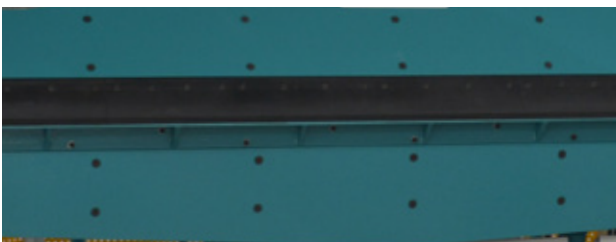
1 Otomatik + 1 Eksen Manuel Arka Dayamalar 1 Automatic + 1 Axis Manual Backgauge 1000mm
