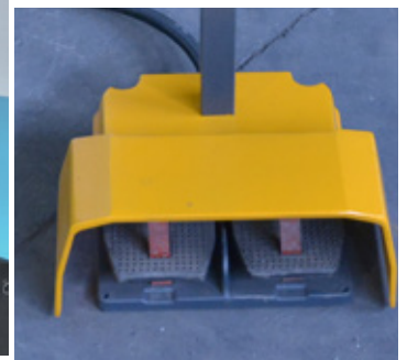
Elleri Serbest Bırakan Ayak Pedalları Handsfree Footpedal Operation for Clamping and Bending
